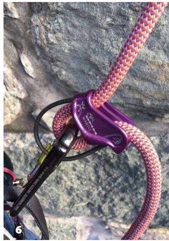
6. Correctly loaded manual braking device [DMM Mantis]. © Libby Peter.
