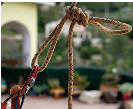
1. Overhand knot with Idiot knot. 2. Mistake of tying slip knot backed up with idiot knot. 3. Slip knot only slips up to the idiot knot. 4. Mistake of threading own-cowstail screwgate. © All photo credits to Rock & Sun Ltd.
